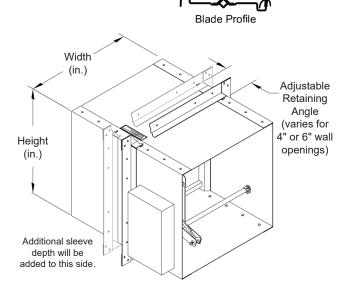
\*Dampers smaller than minimum frame size require a transition. Reference SD-TRFS. Dampers less than 6"H will have a 20" sleeve with the additional sleeve length on the jackshaft side when a B-Pan type transition is ordered.
