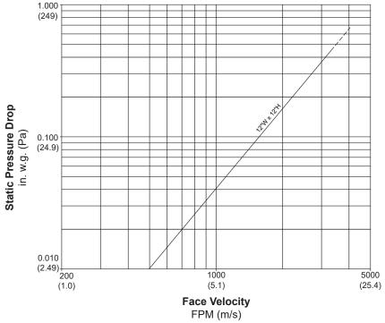
This damper tested in accordance with AMCA 500-D, Figure 5.3
